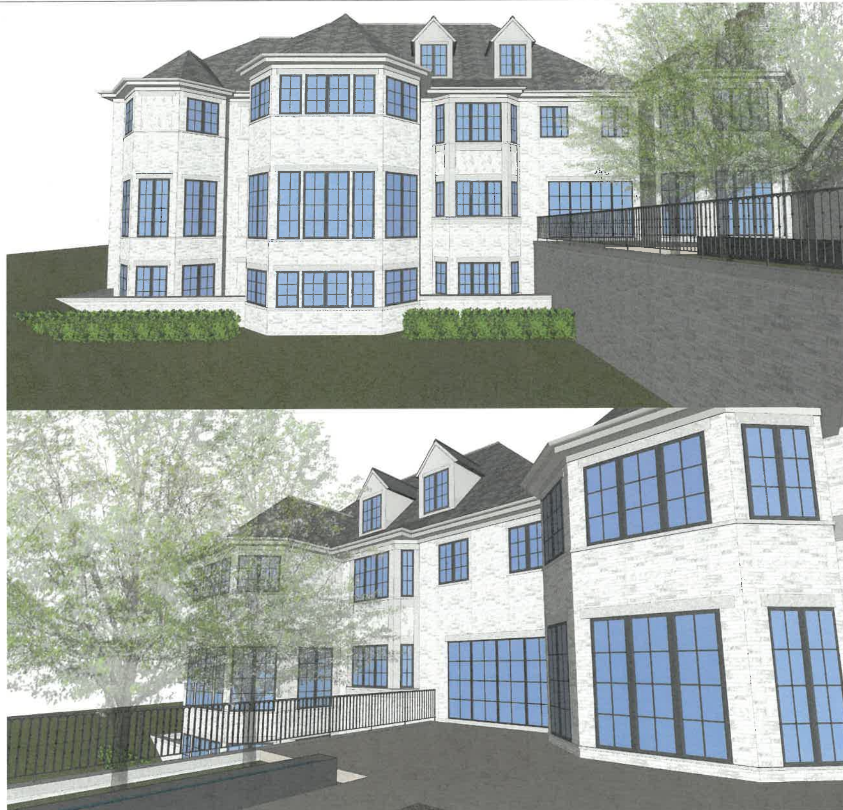
1 REAR ELEVATION RENDERINGS SHOWING REVISED BAY MATERIALS, STEEL AND GLASS ENTRY SYSTEMS, FINAL MARVIN WINDOW CONFIGURATIONS HPC-6 Scale: N/A
