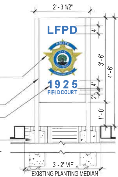
2 PANEL SIGN AT EXISTING MEDIAN 1/2" = 1'-0"
