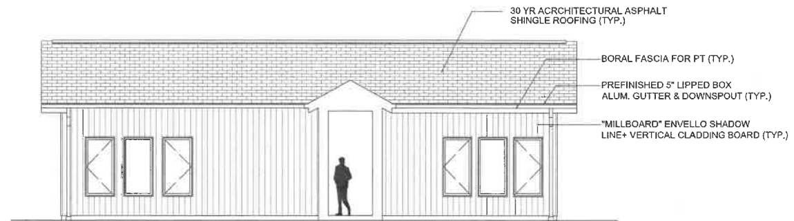
2 EXTERIOR ELEVATION - SOUTH 1/4" = 1'-0"
