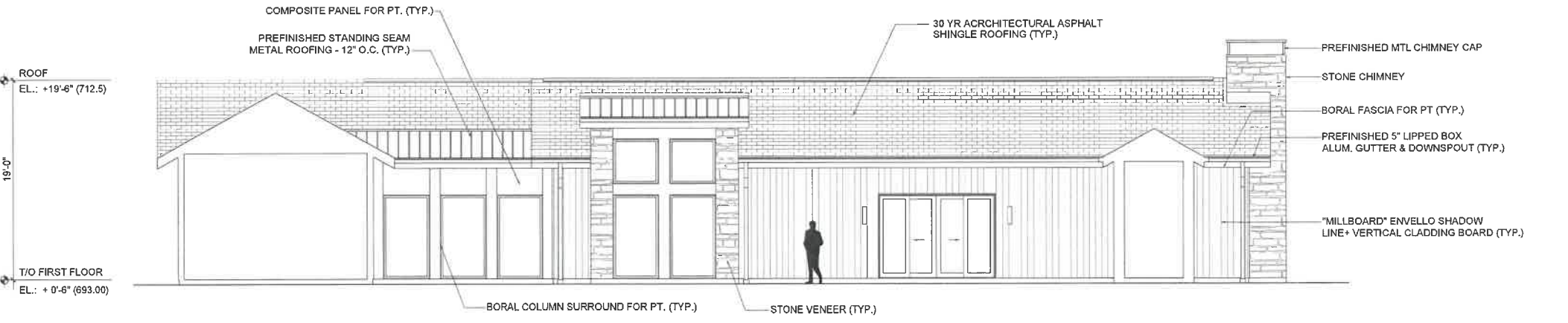
2 EXTERIOR ELEVATION - EAST 1/4" = 1'-0"
