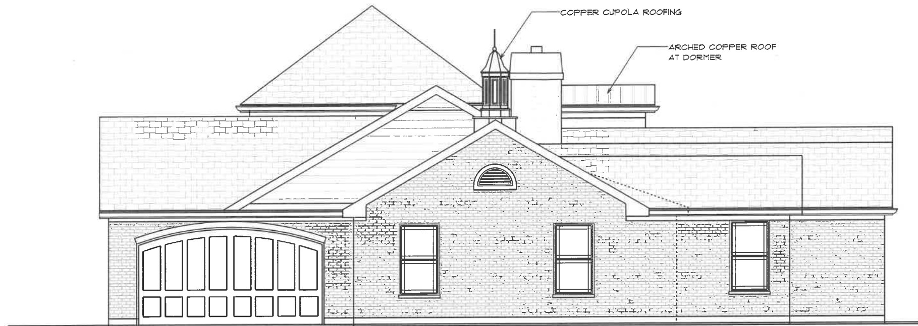
PROPOSED RIGHT ELEVATION SCALE 1/8" = 1'-0"
