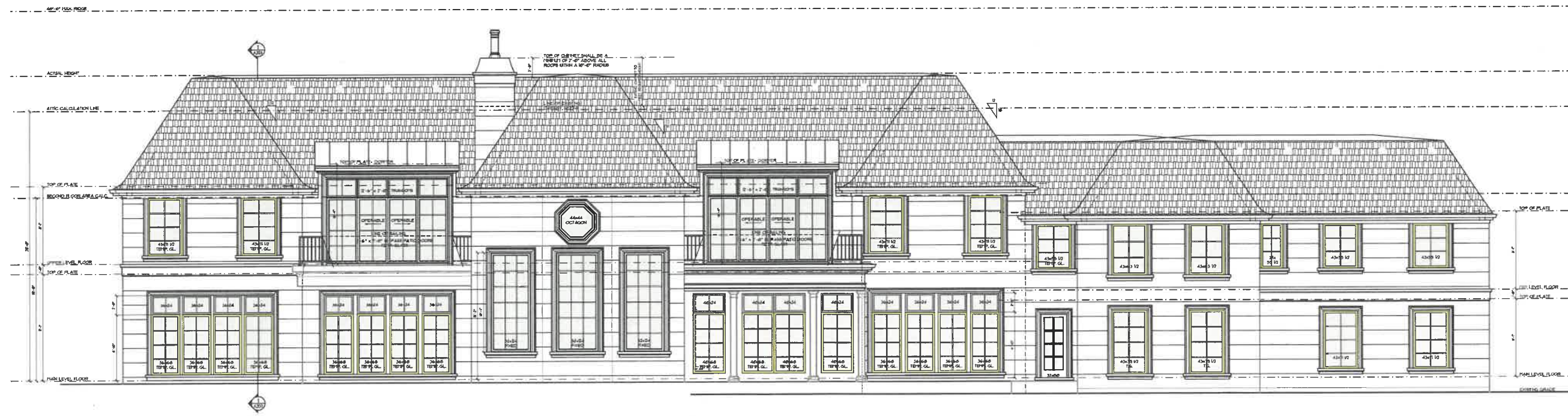
1 New Rear Elevation (Facing East) SCALE: 3/16" = 1'-0"
