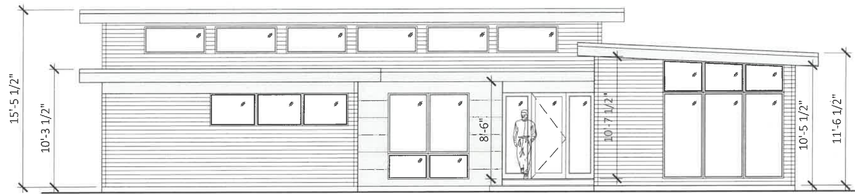
1 NORTH EXTERIOR ELEVATION 1/8" = 1'-0"
