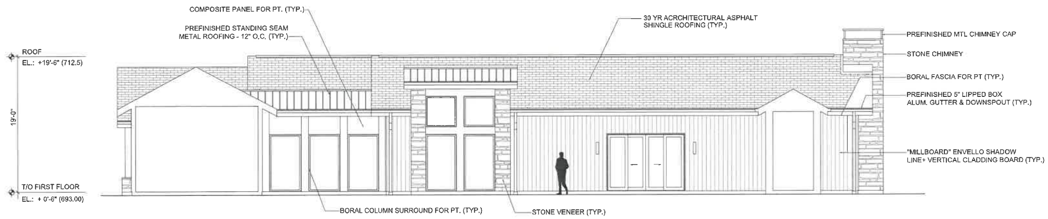
2 EXTERIOR ELEVATION - EAST 1/4" = 1'-0"
