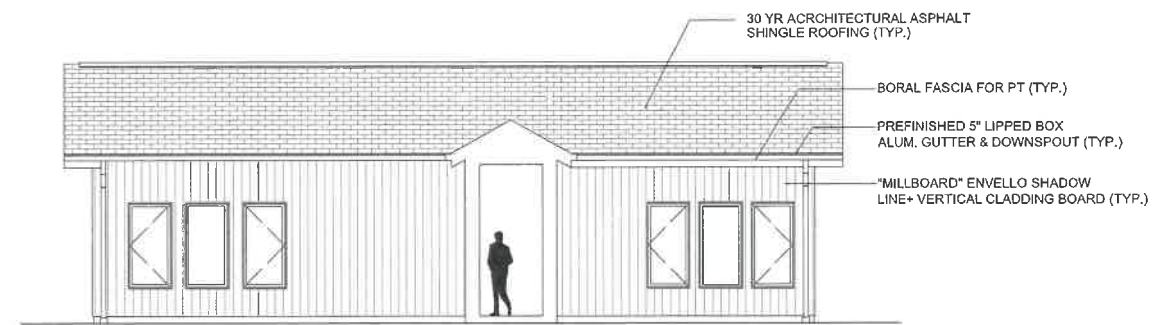
2 EXTERIOR ELEVATION - SOUTH 1/4" = 1'-0"
