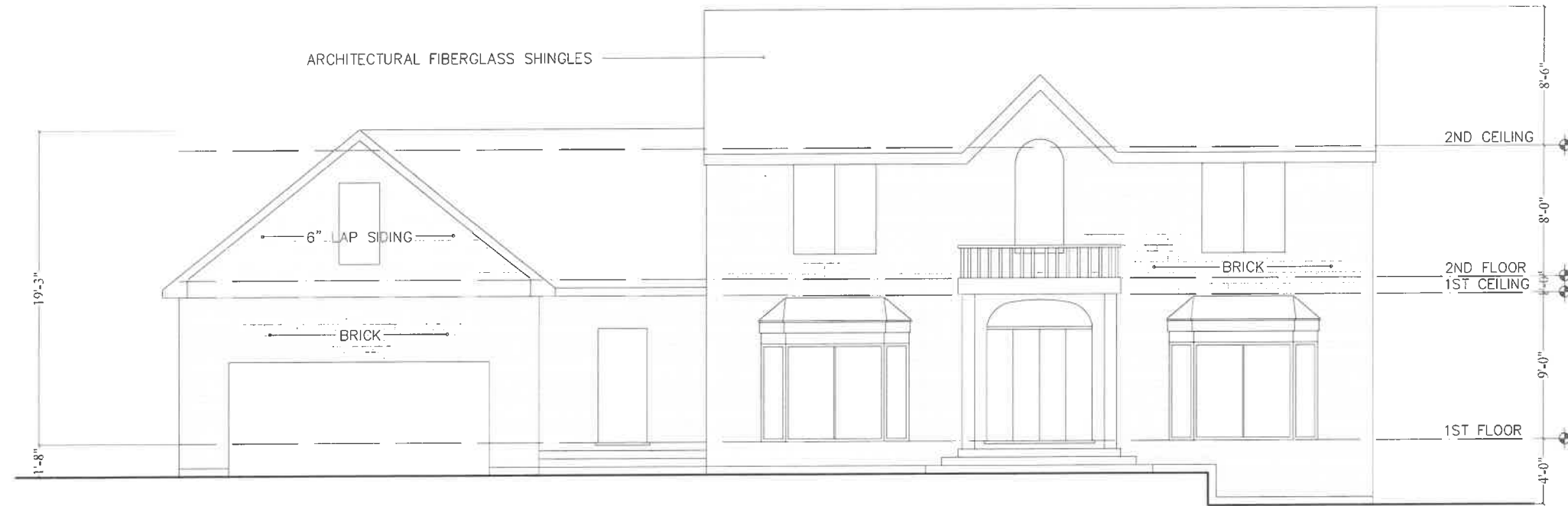
WEST ELEVATION SCALE: 1/4"=1'-0"
