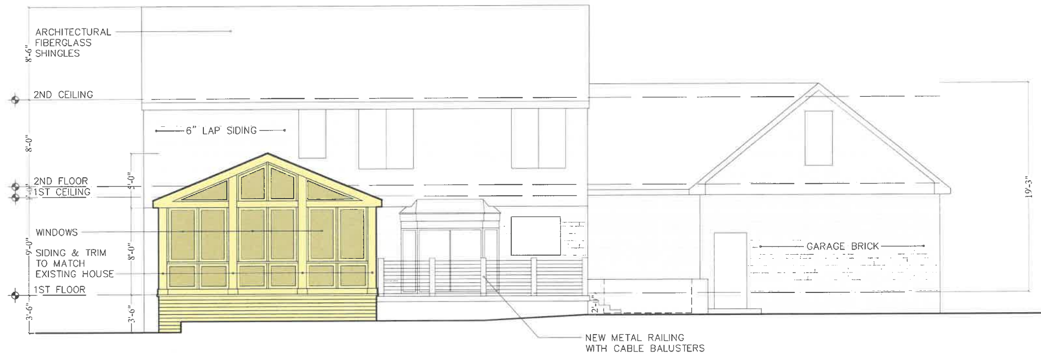
EAST ELEVATION SCALE: 1/4"=1'-0"
