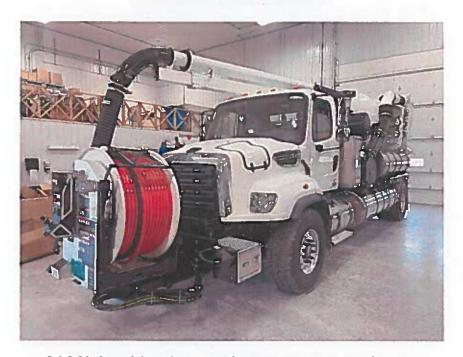
2100i Combination Single Engine Sewer Cleaner with Positive Displacement Vacuum System Mounted on a Heavy Duty Truck Chassis
