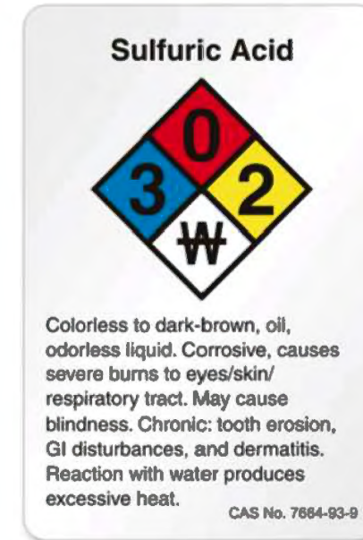
④ NFPA SULFURIC ACID SIGN SIZE: 6.25"x 9" (TO BE MOUNTED ON GATE)
