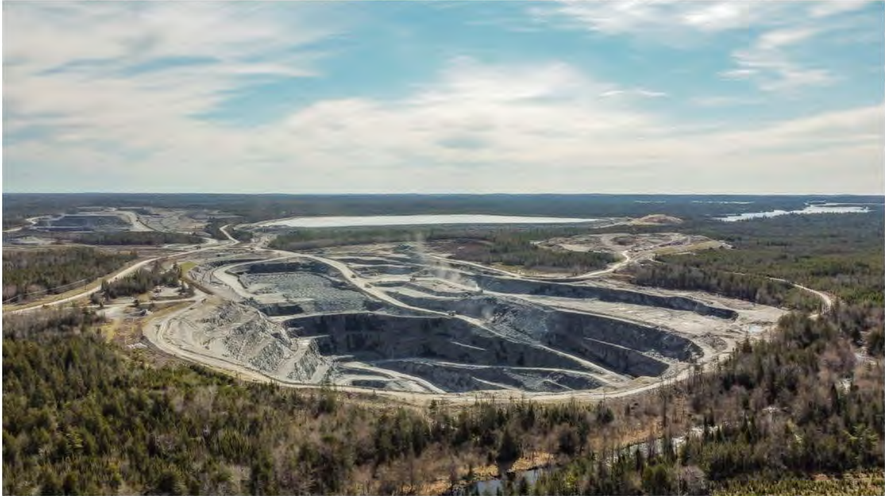
FIGURE 3-5 Open-pit mine at the Touquoy Gold Mine in Moose River, Nova Scotia. The size of this open pit (approximately about 2,000 feet in the longest diameter) is the rough approximate size of open pit that would be used to mine gold from known deposits in Virginia, with deeper ore accessed by underground methods using a shaft or ramp (see Figure 3-4).
