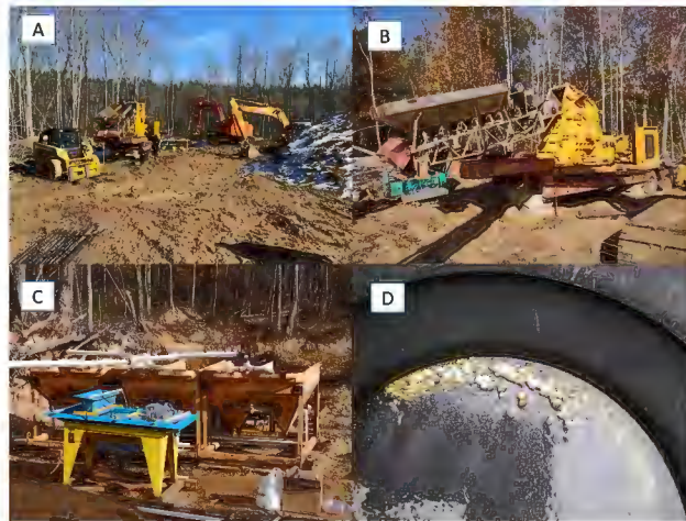
FIGURE 1-5 Photographs of Moss Mine reclamation site, Goochland County, Virginia. (A) Photograph of some of the equipment used to collect rock and sediment materials for reprocessing. (B) Photograph of the crusher being used to process waste material at the Moss Mine. (C) Three jigs used to capture mercury, gold, and lead. (D) Recovered gold and mercury from the Moss Mine site.
