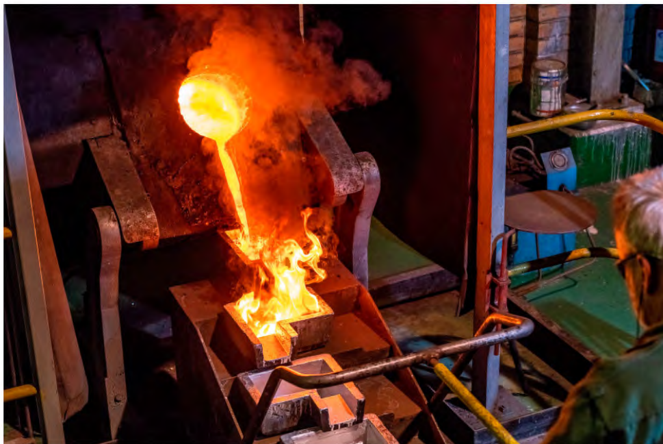
FIGURE 3-19 Doré (gold-rich) metal being poured from a refining furnace. SOURCE: Image by Schoemaker (2022).
