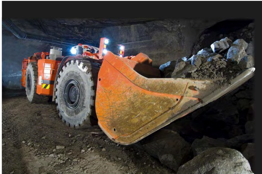
FIGURE 3-8 Load-haul-dump machine used in an underground environment. SOURCE: Image from PJSC Gaysky GOK (2017).
