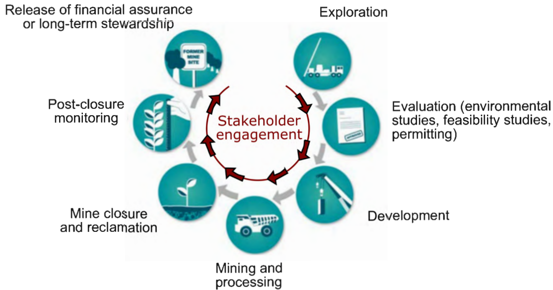
FIGURE 3-1 The life cycle of a gold mine. Stakeholder engagement is a necessary component during all stages of the life cycle and is shown in red, whereas technical, regulatory, and economic considerations by the industry are shown in black.
