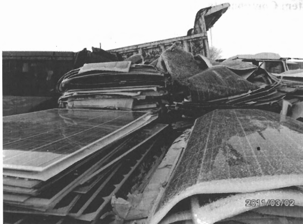
Figure 4: The mangled PV panels in this picture illustrate the nature of broken solar panels; the glass cracks but the panel is still in one piece. Image Source: http://img.alibaba.com/photo/115259576/broken_solar_panel.jpg
