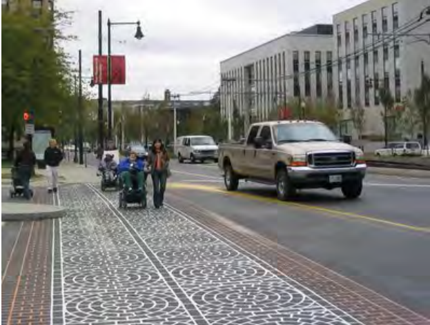
Decorative crosswalks not only define appropriate crossing areas but can also be used as a traffic calming measure.
