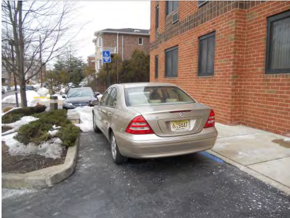
Photo #7: ADA parking without access aisle
