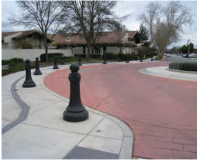
Figure 4.11 DO install special paving and/or bollards to distinguish loading areas.
