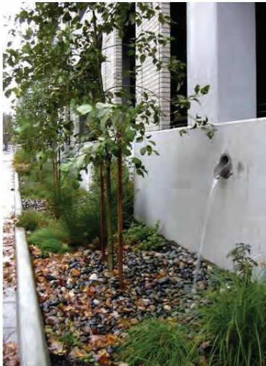
Figure 4.12 DO direct stormwater runoff into permeable areas such as rain gardens.
