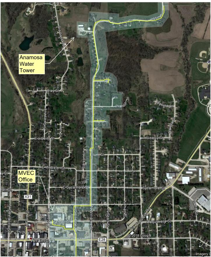
\*\* This map is used for informational purpose of the City of Anamosa, the excavation permit will contain the specific details of the main line fiber installation, the yellow line represents the route of the fiber the white shaded area indicates the approximate areas that MVEC will offer FTTH service to\*\*
