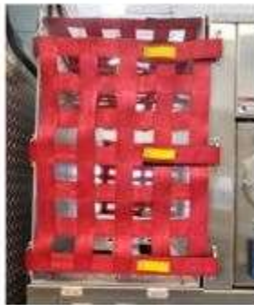
Footman loops may be on sides, bottom Or combination of both depending on Apparatus design
