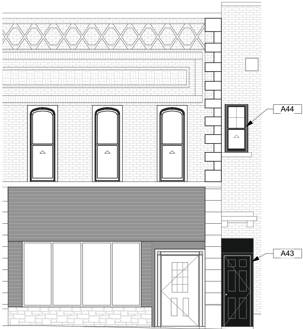
EXTERIOR ELEVATION - COLOR SCHEME 3/16" = 1'-0"
