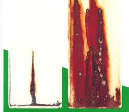
One cost of Series 91-H,O Hydro-Zinc, then two costs of Standard three-coats of the component exert.
