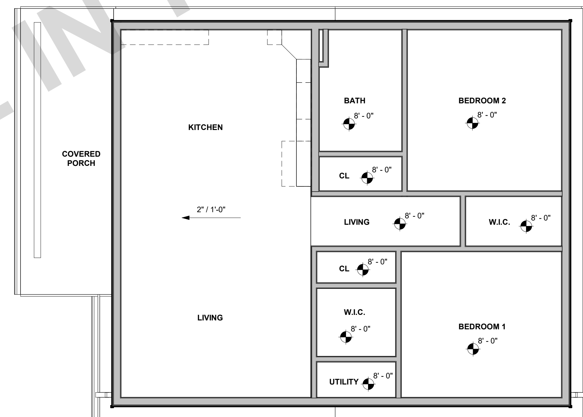
3 GROUND FLOOR RCP - CALIFORNIA RANCH A1-201 | A3-121 SCALE: 1/4" = 1'-0"
